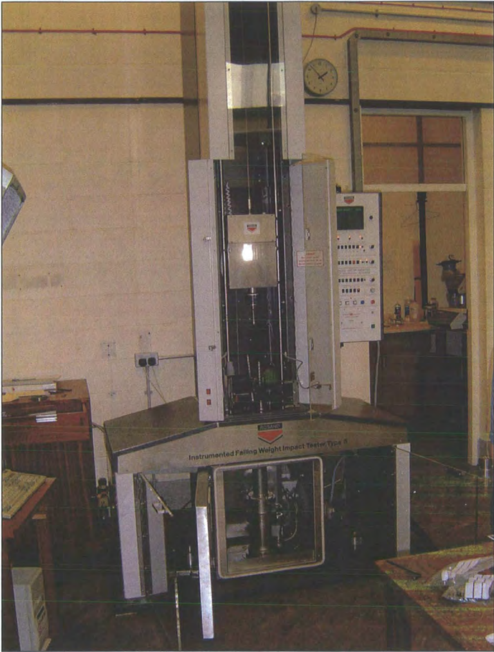
Figure 4.13 Rosand Type 5 Falling weight impact tester
