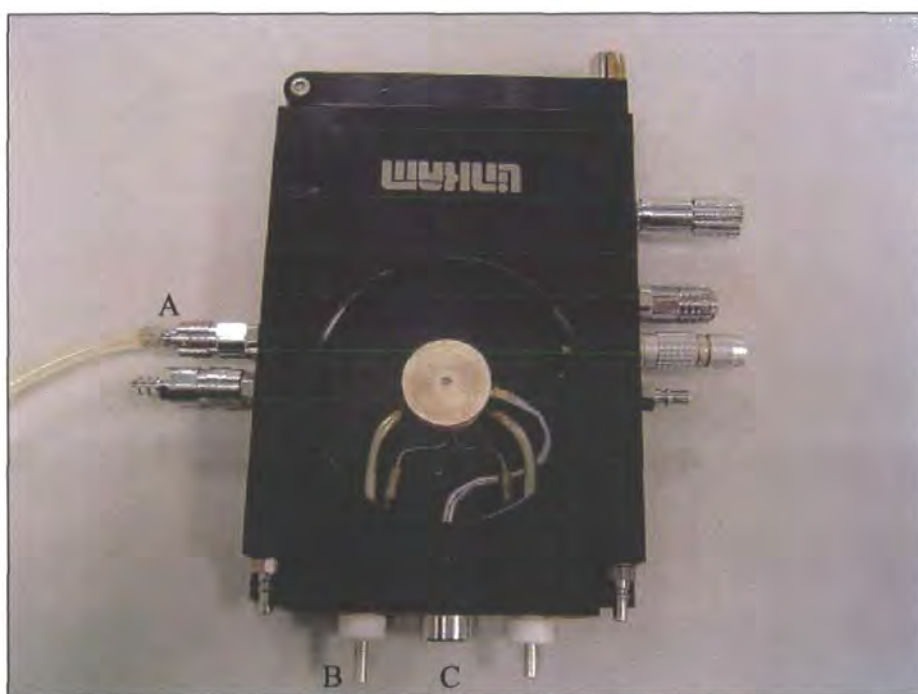
Figure 2.24 Linkam hot stage used for OM, N 2 (g) supplied via “A”, cold N 2 (g) supplied via “B”, power supplied via “C”
