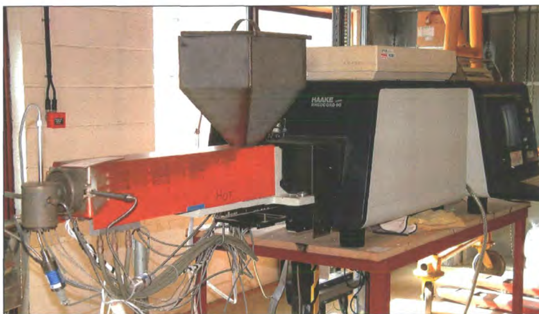
Figure 2.22 Haake Rheocord used for melt blending PET and PC on kilo scale
