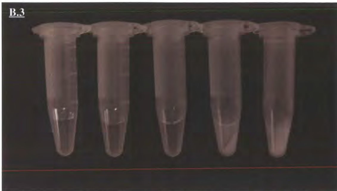
Fig:6.4 B.3: Samples as per Fig:6.14. The reduction of the pH level to 9 with 1 M HCl caused precipitation of a white solid. More solid was visible in the more concentrated amino-G solutions
