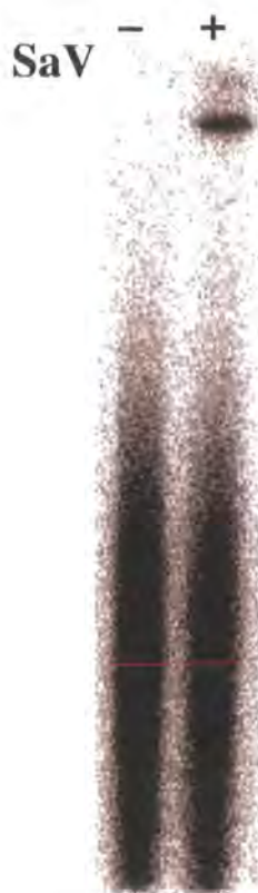
Fig:7.10 IP image of a PAGE gel showing the results of a streptavidin assay. The two lanes were both loaded with 5'-Azido-RNA that had been subjected to a CuAAC bioconjugation reaction, only one lane however also contained streptavidin in the buffer.
