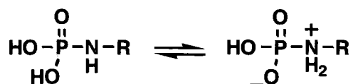
Fig:2.15 The two forms of neutral phosphoramidates, the non-zwitterion (left) and zwitterion (right) species. The high rate of phosphoramidate solvolysis (see Fig:2.7) at low pH was attributed to the instability of the zwitterionic species.
