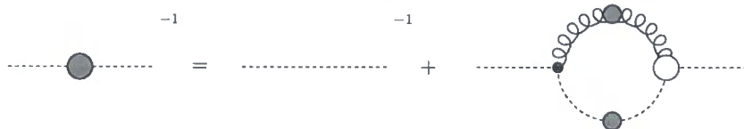
Figure 4.3: The quenched ghost SDE. Filled dots indicate full propagators and vertices. Dashed lines indicate ghosts, whilst wiggly lines represent gluons.
