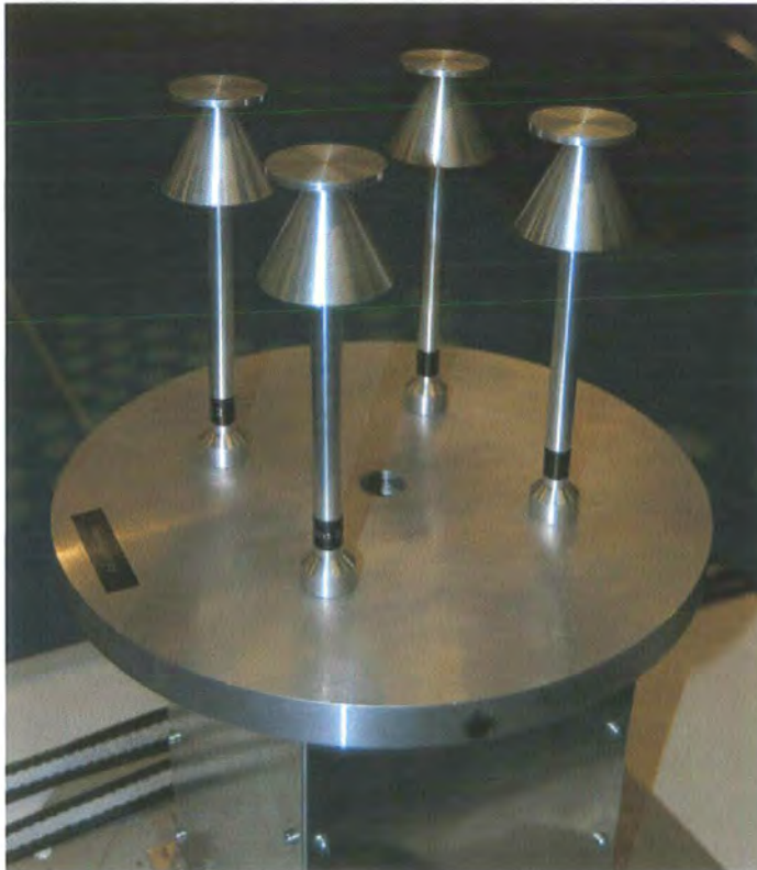
Figure 6.27: Wideband (2-6 GHz) Discone circular array (showing 4 elements) [28].
