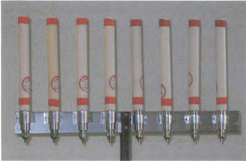
Figure 6.28: Omni-directional dipole linear array (showing 8 elements). This array is nominally working at UMTS frequencies.
