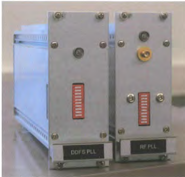
Figure 6.16: Photo of the PLLs used in the sounder.
