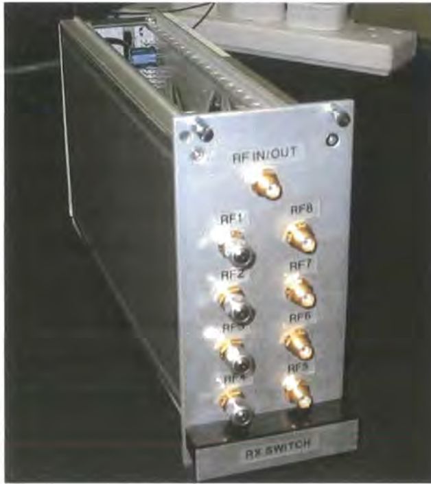
Figure 6.13: Photo of 8-way RF switch.
