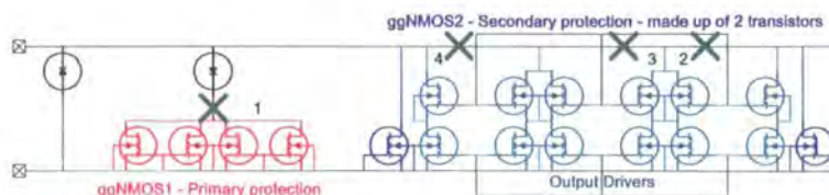
Figure 3.24: Output circuit of the BC01b showing the location of the FIB cuts to be done
