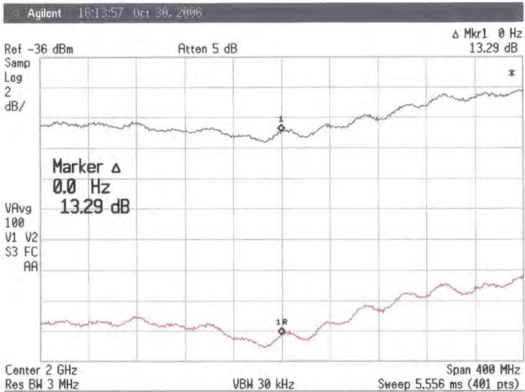
Figure 5.15 “y-factor” measurement of the 3.5 GHz down-converter
