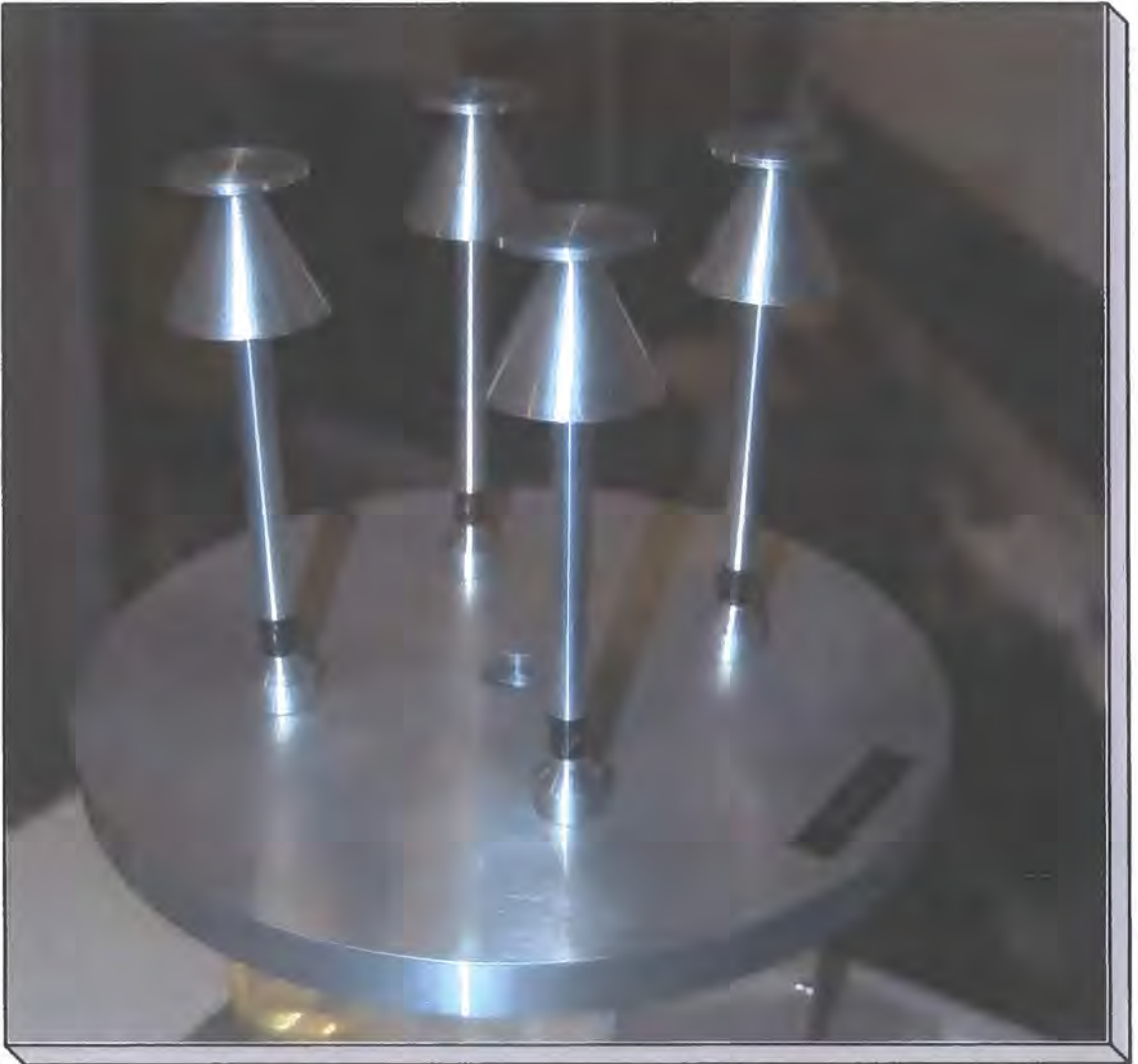
Figure 4.57 Array of 4 discone antennas operating at 2.3 and 5.7 GHz simultaneously
