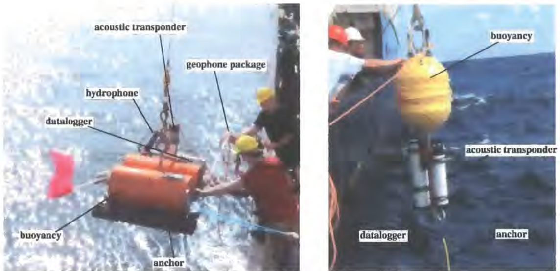
Figure 3.1: Deployment of an OBS (left) and OBH (right). Both instruments consist of a large, brightly coloured buoyancy device, an anchor, a datalogger, an acoustic release transponder, an hydrophone and, in the case of the OBS, a deployment arm and 3-component geophone package.
