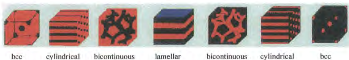
Fig. 1.18 Self-assembly structures for a block co-polymer. (after Floudas G, et al. , Macromolecules 2001 34 2947)
