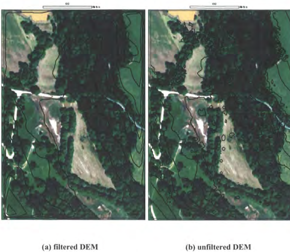
Figure 4.6 5 m interval contour map derived from the filtered 5 m LiDAR DEM (a) and the unfiltered 5 m LiDAR DEM (b) in the flood model test area
