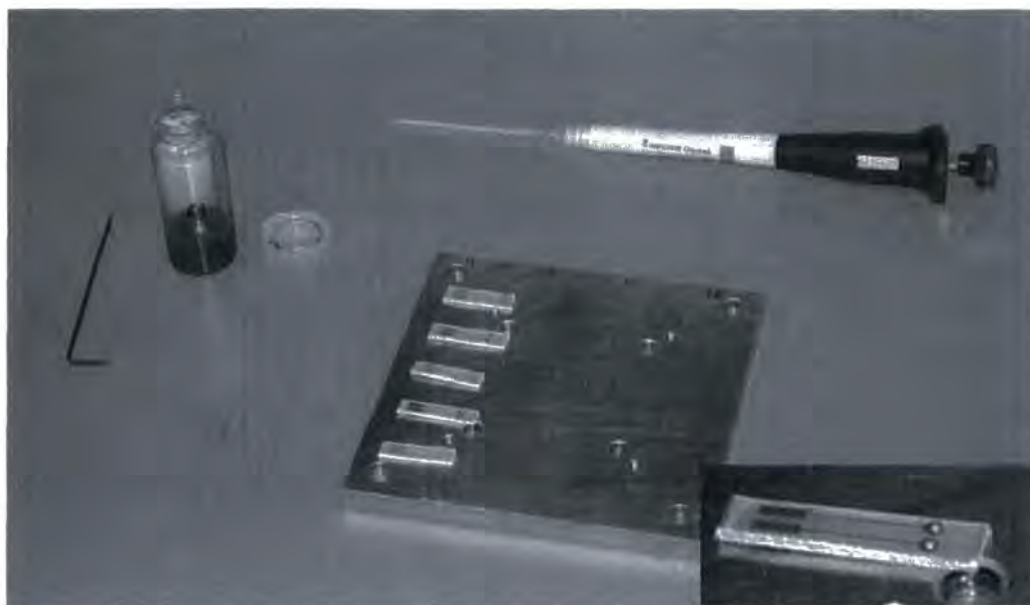
Figure 5.3: Sample boards and positive displacement dropper, insert shows electrode.
