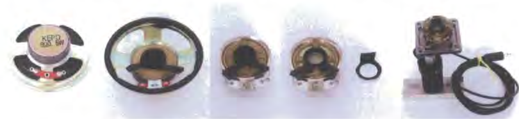
Figure 8.24: A series of photos showing various stages of constructing a laser shutter made from a speaker coil.
