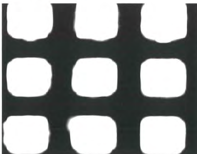
Figure 23: A fluorescence micrograph of a cresyl violet perchlorate tagged pulse plasma polymerised pattern of glycidyl methacrylate on a polytetrafluoroethylene substrate
