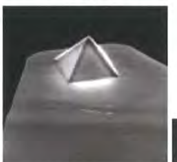
Figure 8: An AFM tip, an inverted pyramid of 3 \mu\text{m} height and 10 nm tip radius, usually made with Si or \text{Si}_3\text{N}_4 e . Scale bar is 3 \mu\text{m} .
