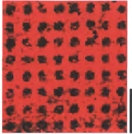
Figure 31: Fluorescence micrograph showing non-fluorescent spots of polybutadiene exposed after lift-off of an acrylic acid pattern and plasma polymerisation of glycidyl methacrylate
