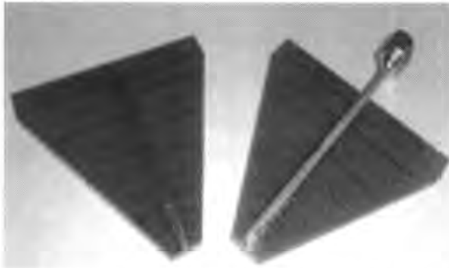
Figure 4.3: Log-Periodic Antennas (900-2600 MHz) [4]
