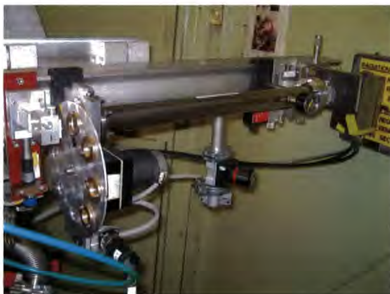
Figure 3-5: SRS Station 2.3 detector arm assembly showing the anti scatter slits, attenuator, evacuated beam path, detector slits and detector.
