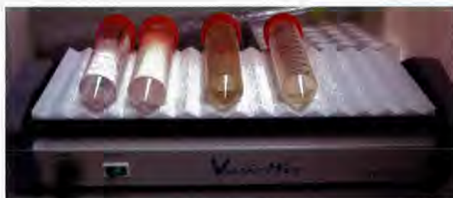
Fig. 3.4 Shows the 50 mL centrifuge tubes containing the aqua regia, MQ H 2 O and the CCl 4 , on the shaker.
