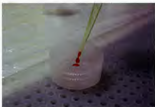
Fig 3.5 Shows the chromium oxide ( \text{Cr}_2\text{O}_3 ) being added to the 12N sulphuric acid ( \text{H}_2\text{SO}_4 ) droplet in the rocket vial lid. Fig. 3.6 Shows the rocket vial upside down and sealed with the hydrobromic acid (HBr) droplet in the bottom of the cone, and the chromium oxide and sulphuric acid in the lid.
