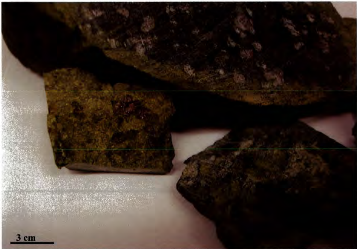
Fig. 2.3 Sample 474538 (on-craton) of the W.G. peridotite suite. This sample shows clearly the orange weathered surface and the grey-black fresh interior. Millimetre sized garnets are visible on the weathered and the freshly cut surface.
