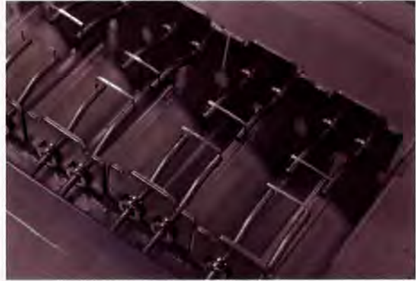
Fig. 3.10 Shows the filaments with their welded Pt ribbons, ready for the Os loading procedure.
