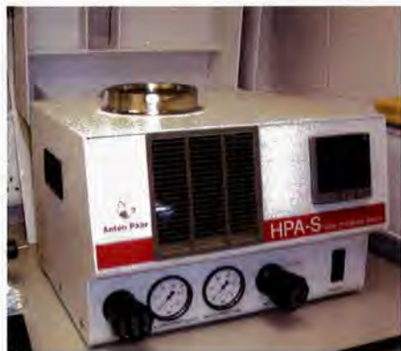
Fig. 3.2 The Anton Paar-Perkin-Elmer high pressure asher (HPA-S).
