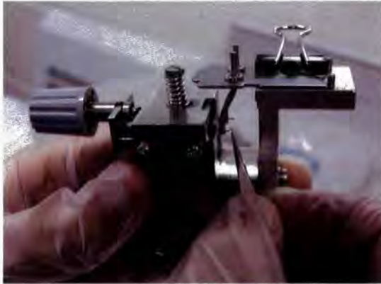
Fig. 3.9 Shows the Pt ribbon being welded onto the filament
