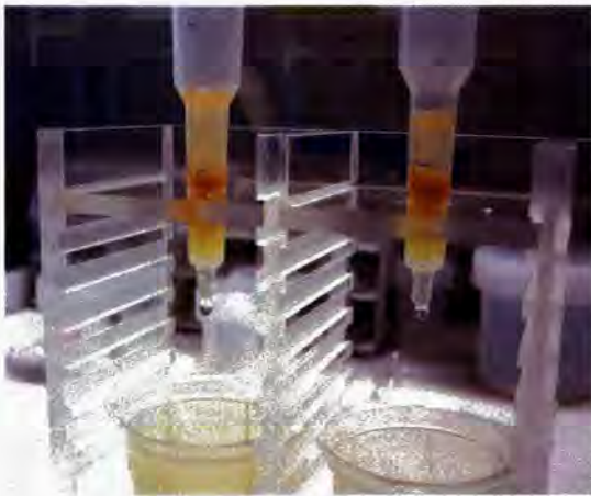
Fig. 3.8 Photo taken in the clean lab, of the PGE column chemistry. The orange colour in the columns is the resin. Acid is dripping through the columns into the waste beakers below.
