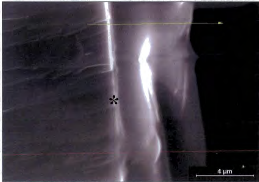
Figure 4.4 – ESEM image of the standard formulation dried size film: Yellow arrow = area investigated by X-ray analysis; * = to the glass-film interface.
