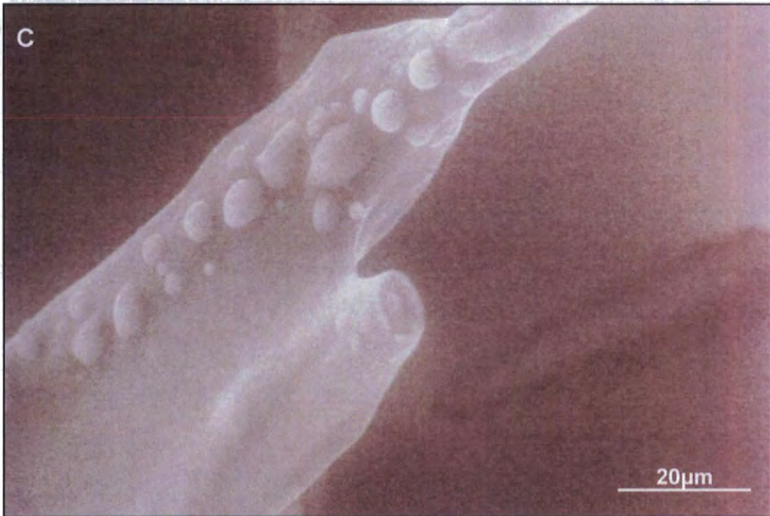
Figure 5.20 – Images showing initial stages of wetting of newly sized glass fibres
