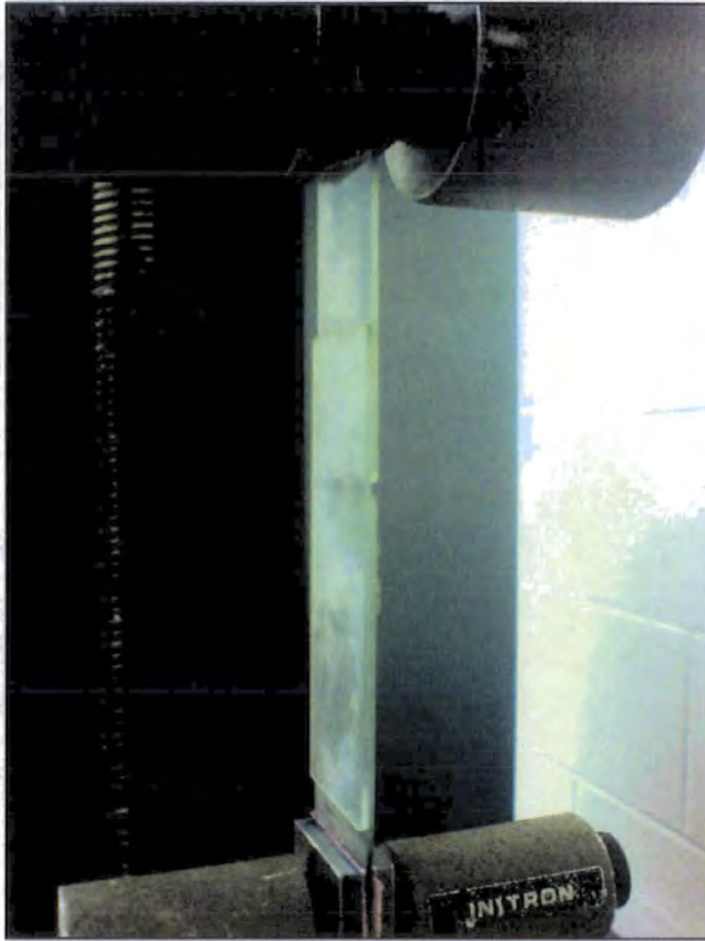
Figure 3.8 – Image of the lap shear test being run on the pyramid sample
