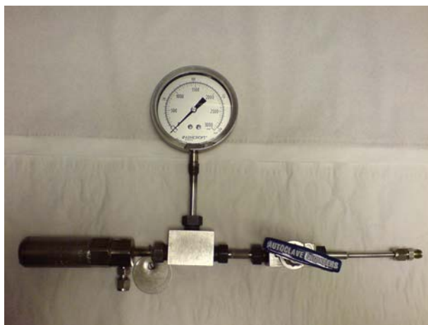
Figure 17. Autoclave vessel (25cm 3 ) used for high pressure reductions of alkenes
