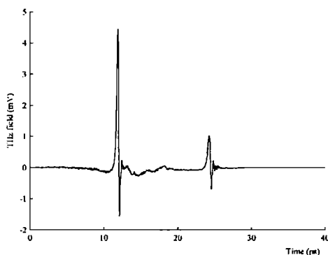
Figure 4.18: Smoothed THz reflected waveform.
