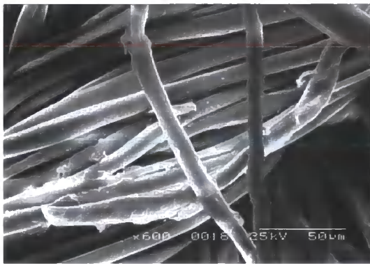
Figure 3.9: Magnified SEM of one (shirt) yarn.
