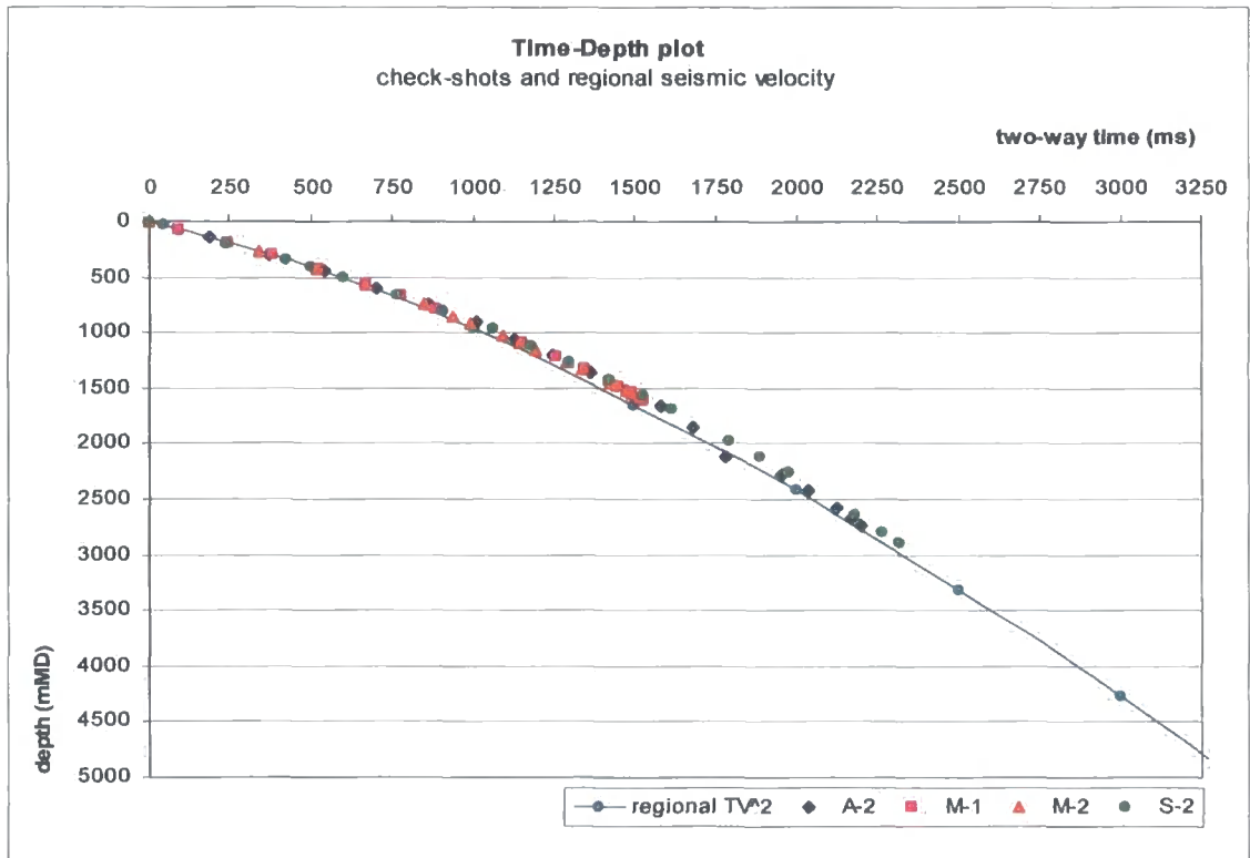
Figure 3.6b Graph showing the check-shot data plotted with the regional velocity function (solid curve) used to process the seismic data. In both cases, the velocity is shown to increase with depth. There is a reasonably good fit between the seismic velocity curve and the check-shot data; however, between c. 1500 and 2400m MD the predicted velocities are slightly higher than those obtained from the check-shots.
