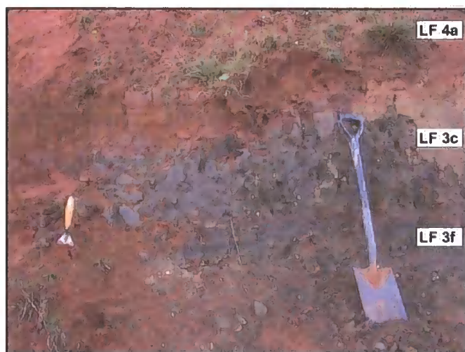
Contact between LF 4a and LF 3c with laminated diamicton (LF 3f).
