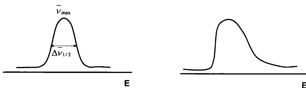
Figure 1.4 Representations of typical optical transition bands illustrating the ‘cut-off’ observed for Class III complexes
