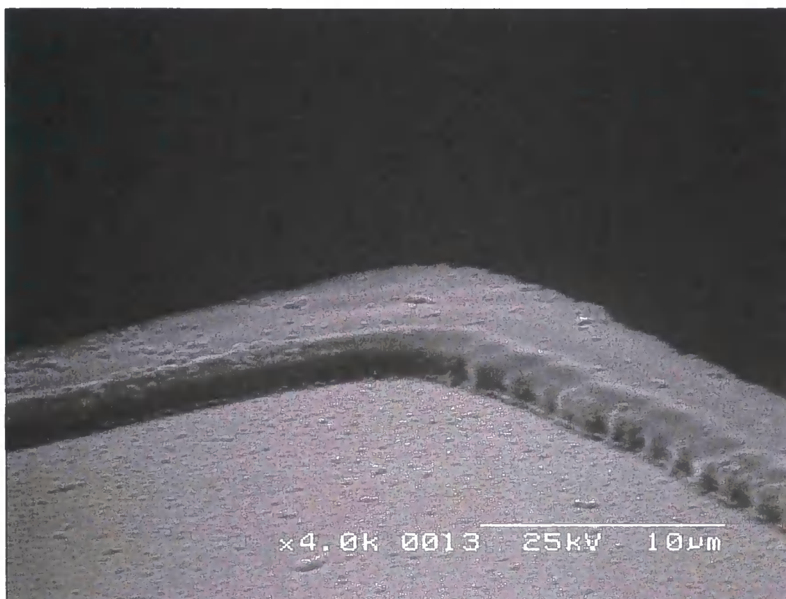
Figure 5-13 Metal contact pads overlapping edges of SU-8
