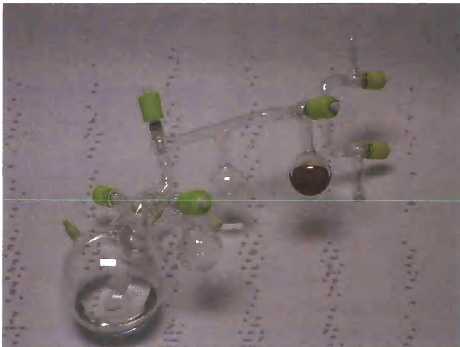
Figure 6.1 Christmas tree vessel used for anionic polymerisation.
