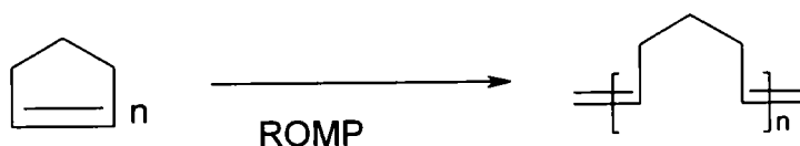
Figure 1.7 ROMP polymerisation showing the alkene incorporation into the polymer backbone.
