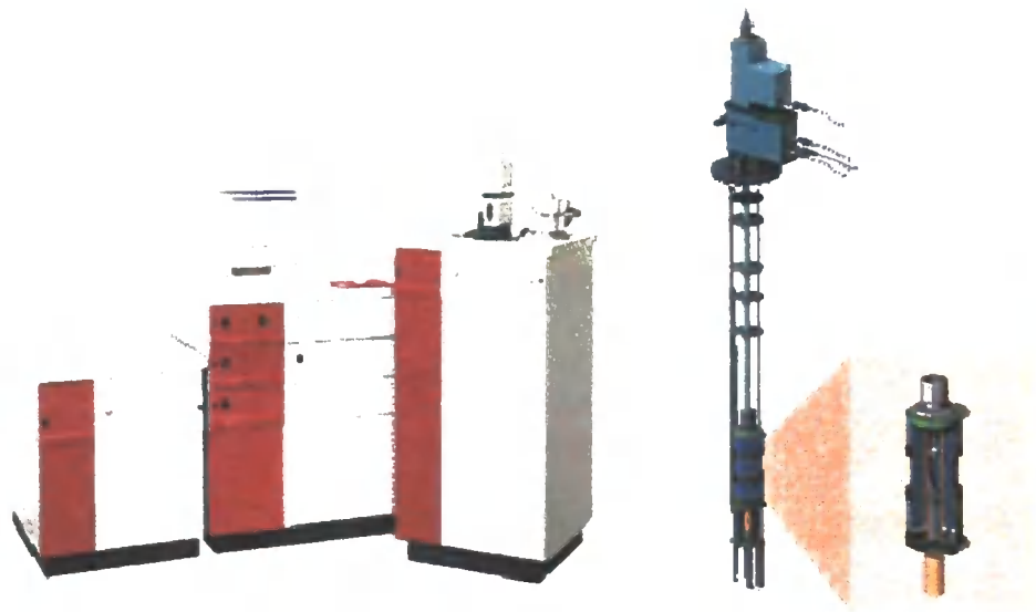
Fig. 2.5. The picture of whole MPMS components (left), schematic diagram of MPMS probe with blow up of superconducting solenoid detector coil (right).
