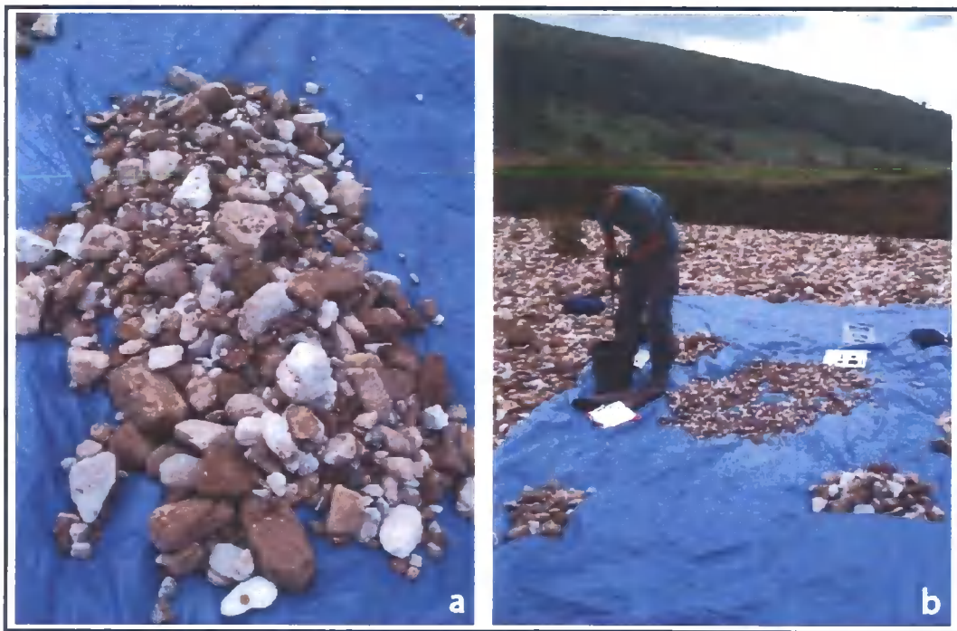
Figure 5.7: Photos taken at site 350 showing (a) the bulk sample and (b) coarse sediment sorted into piles, then weighed in the bucket using a spring weight.
