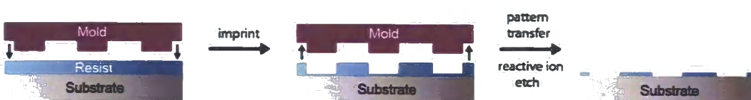
Scheme 2. Schematic of principle processes used in NIL.
