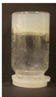
Figure 5.10: Metallogel formed from 5.14 and silver(I) nitrate.
