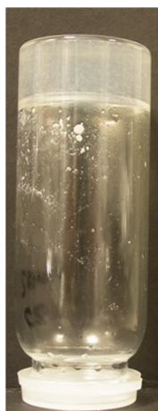
Figure 5.16: Metallogel formed from 5.12 and silver(I) nitrate in water and THF (2:3).
