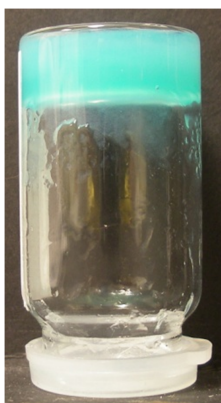
Figure 5.3: A copper(II) chloride gel formed with 2.1 .
