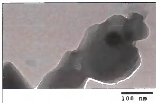
Figure 4.25 TEM image of the dry Ni 2 TCNQ sample displaying chaining.
