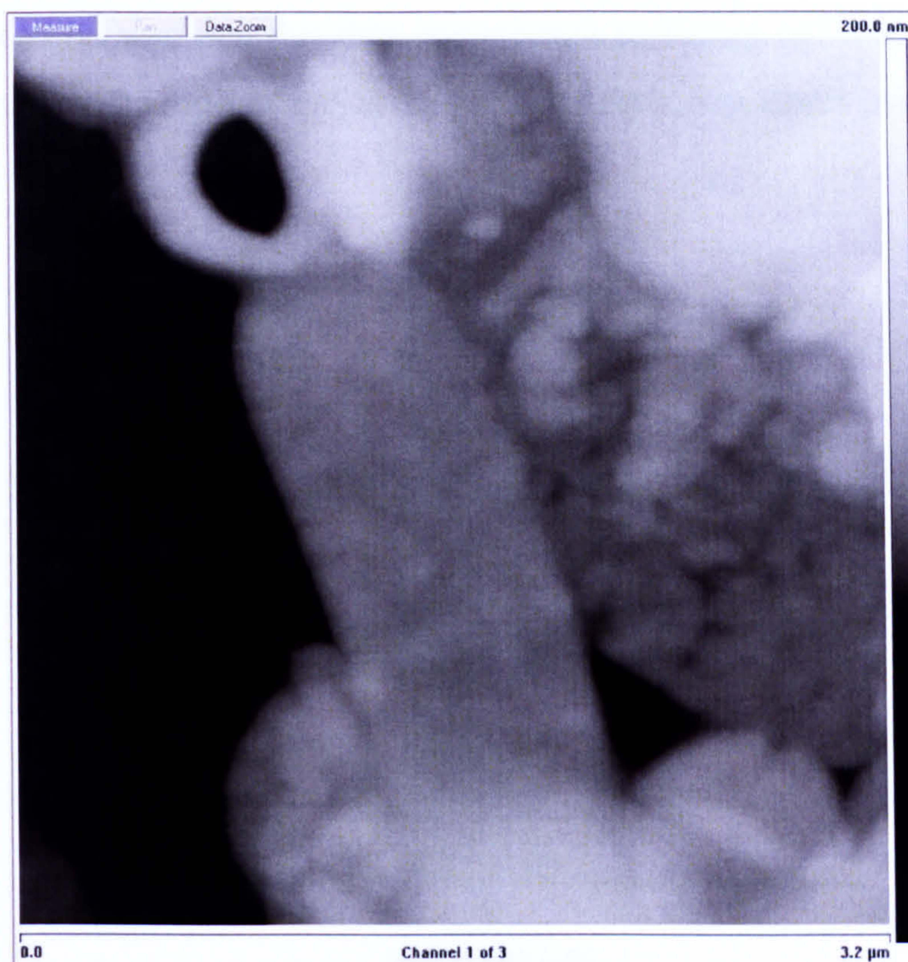
Figure 119 a high magnification image of the PEEK particles from the PEEK on ceramic simulator test
