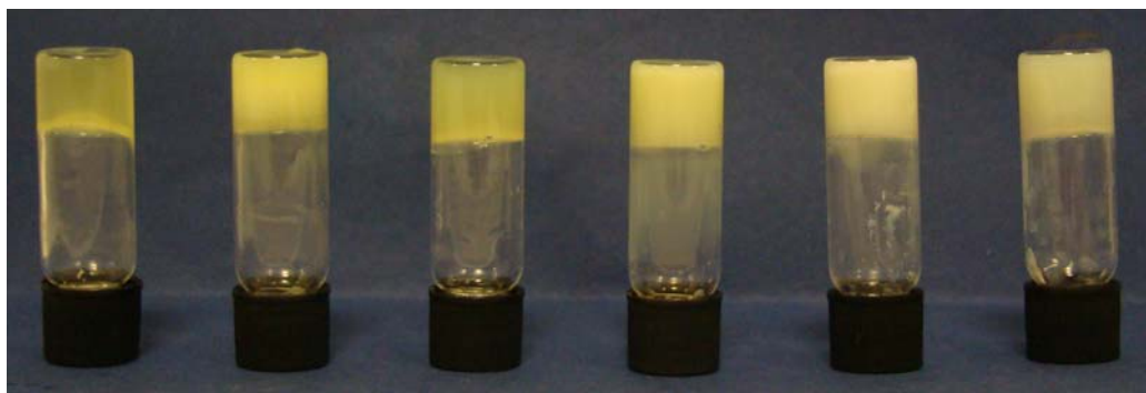
Figure 3.62. Photograph of gels of 3.10 at 1% by weight in water acidified with, from left to right, EtPO 3 H 2 ; MePO 3 H 2 , H 3 PO 4 ; H 2 SO 4 ; HPF 6 and HBF 4 . The samples for the acids H 3 PO 4 ; H 2 SO 4 ; HPF 6 and HBF 4 are the same as those shown in Figure 3.31.
