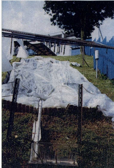
Figure 3.25 Calibration of the rainfall simulator for different sets of sprinklers for the production of different rainfall intensities.
