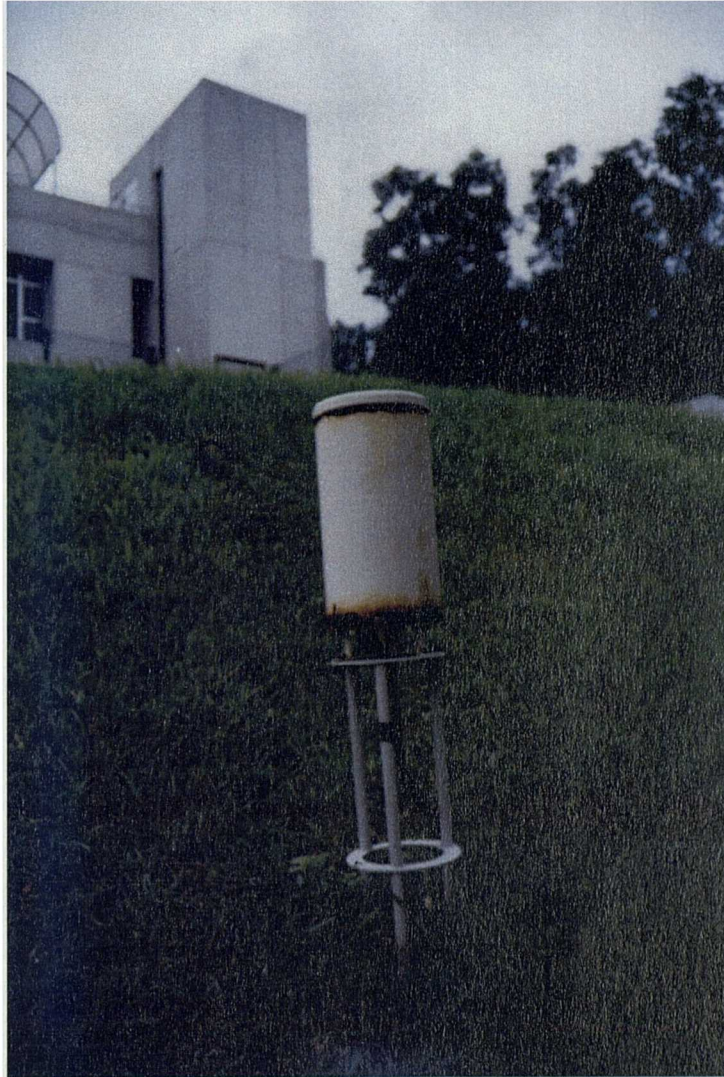
Figure 3.15 Handar double tipping bucket rainfall gauge that is installed on the NTU-CSE slope.
