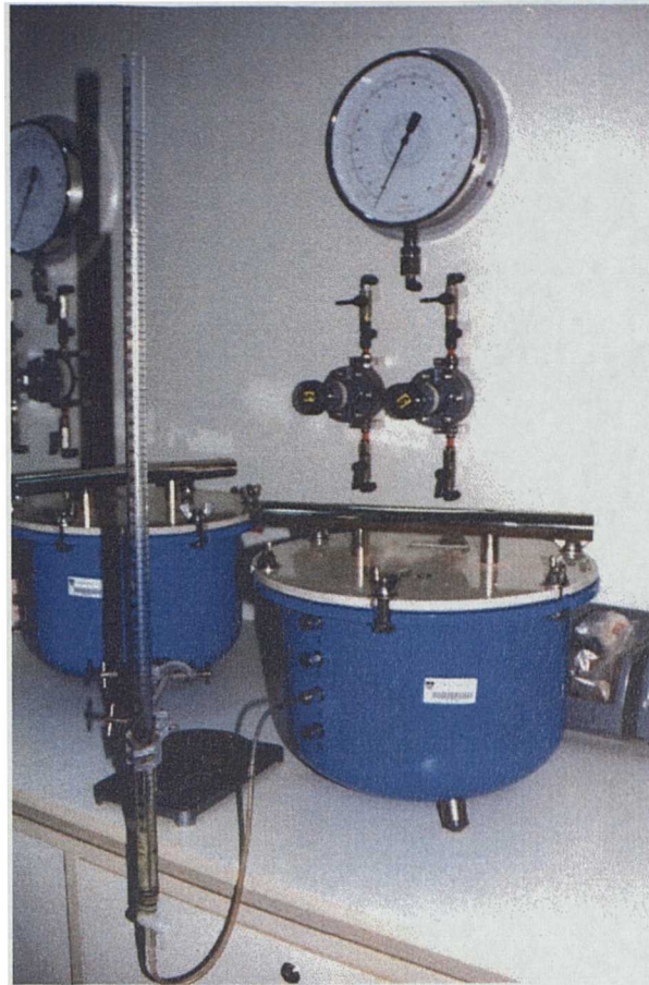
Figure 3.30 The 1600 model pressure plate, manufactured by Soilmoisture™ Equip., Santa Barbara, California.
