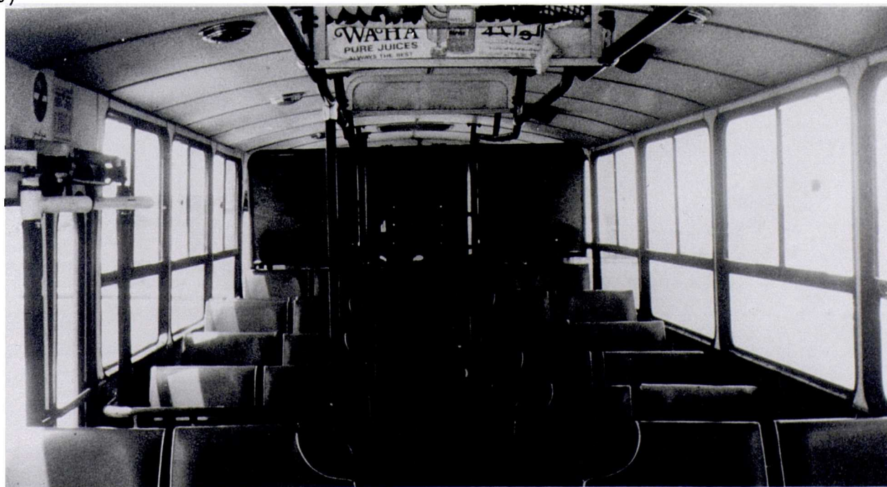
Interior of a SAPTCO bus showing rear partition used to make a segregated female compartment.
