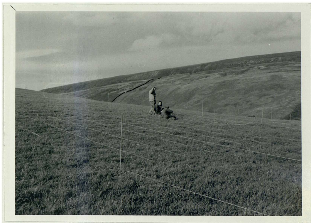
PLATE 3 - Sampling grid used for study of methods of grassland survey, Keld, Upper Swaledale
