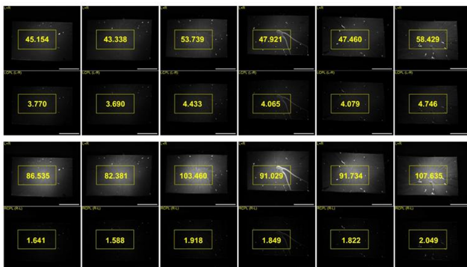
Figure S12: CPLP of six sequentially spin coated PMMA films containing \Delta -EuL using BPF594/10 (top two rows) and BPF610/10 (bottom two rows) where L+R (1 st and 3 rd rows) and L-R (2 nd and 4 th rows) with regions of interest for g_{\text{CPLP}} calculations and their average intensities shown in yellow. Scale bar = 5 mm. R-L and L-R images are 6 times contrast enhanced for display.
