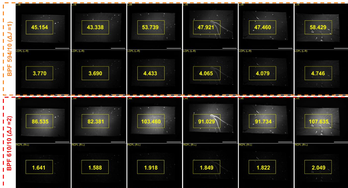
Figure 4.10: EDCC images of six sequentially spin coated PMMA films containing \Delta\text{-EuL}^1 using BPF594/10 (top two rows) and BPF610/10 (bottom two rows) where L+R (1 st and 3 rd rows) and L-R (2 nd and 4 th rows) with regions of interest for g_{\text{CPLP}} calculations and their average intensities shown in yellow. Scale bar = 5 mm. R-L and L-R images are 6 times contrast enhanced for display.
