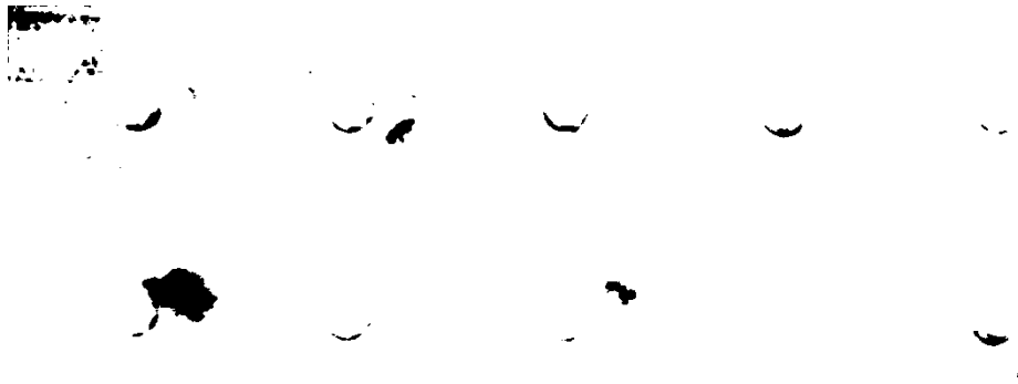
Figure 22: The image after the performing thresholding the first time, with all areas above a value of 140 being set to white, and all others to black
