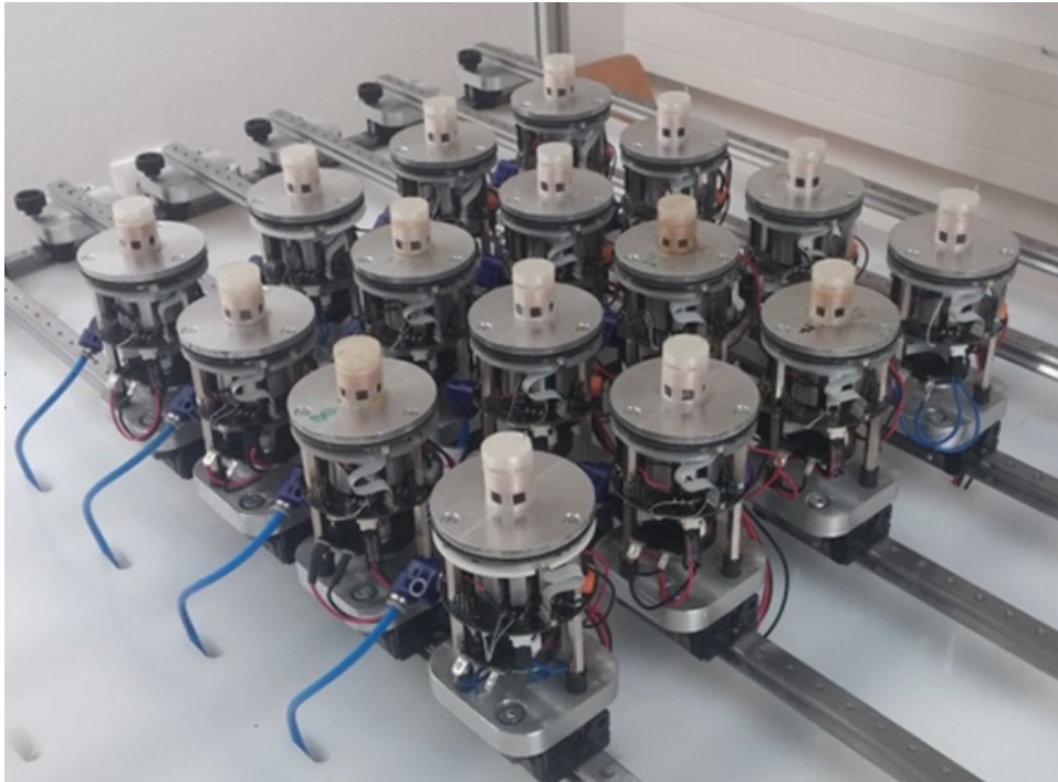
Figure 13: An array of CASUs, as used in the ASSISI arena, mounted on rails without any wax sheets covering them, from [99].
