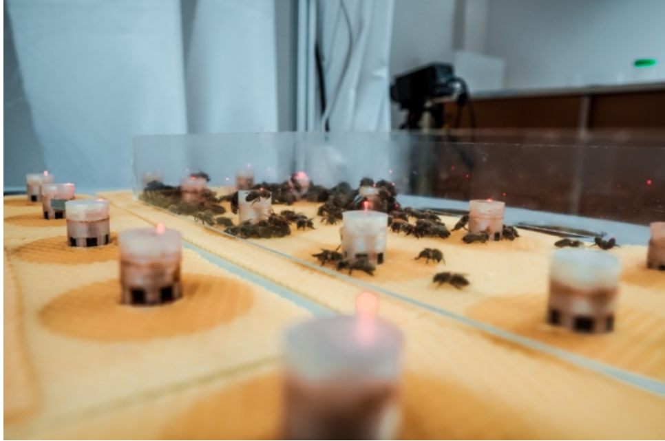
Figure 12: A picture of the ASSISI arena, with bees present. Only a small part of each CASU unit is visible above the arena, containing its components to create a stimulus. Also not the wax sheets covering the units.
