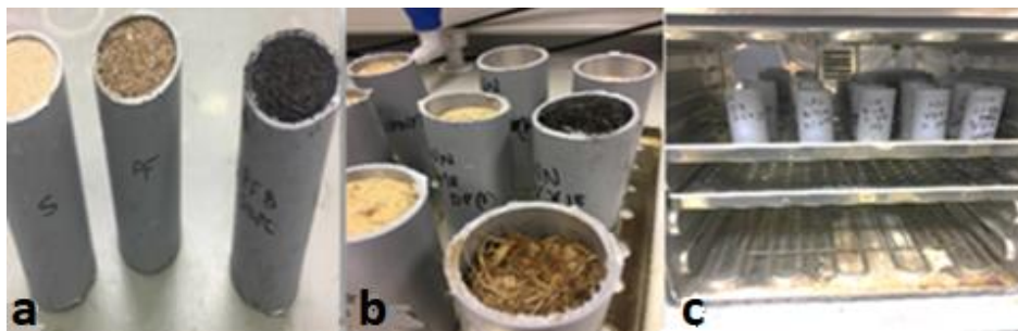
Figure 3.2. (a) shows the 3 materials used, which are: Sand, DPF and biochar. (b) shows the treatments of biochar and DPF. (c) The samples were placed on a tray, then in the oven for 3 weeks at 40° C.
