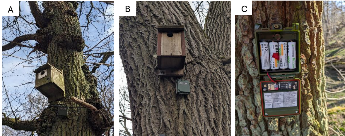
Figure 2.4, Recording Equipment In-Situ. (A) Audio recorder secured to a tree using a locking strap. (B) Audio recorder mounted to a tree using screws. (C) Internal view of the recording device, showing component layout.
