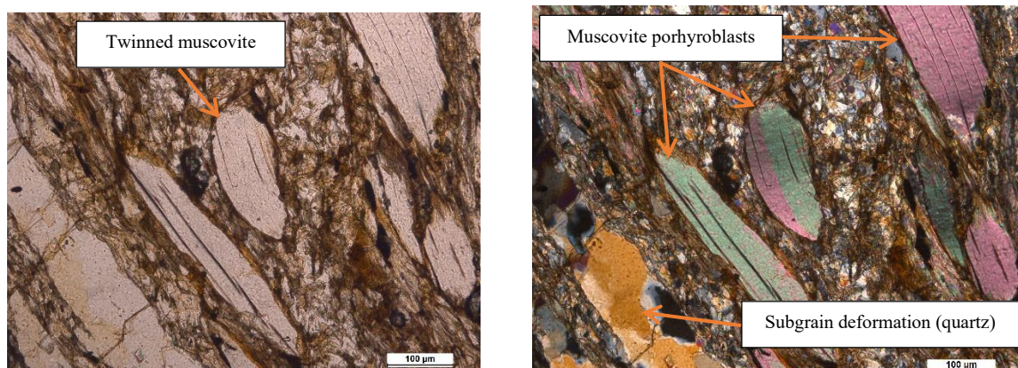
Figure 4.37: PPL (left) and XPL (right) of 1.AS.4 (80µm Section). A closer look at a quartz vein (bottom left) and muscovite porphyroblasts. In the centre, a muscovite porphyroblast is twinned along its basal plane (001).
