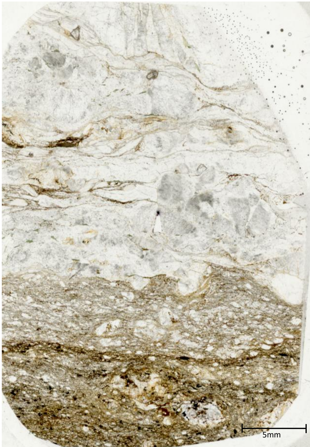
Figure 4.27: 1.AS.MP.B 80um Thick Section Scan. Significant contrast from the relatively biotite-enriched Alpine Schist to the quartz-feldspar dominated Mataketake Pegmatite. Note the absence of biotite streaks in the pegmatite. Microscopy identifies muscovite-dominated streaks in the pegmatite. The most notable change apart from colour, is grain size. Large porphyroblasts of feldspar and muscovite are deformed. The former show bookshelf fracturing, and kink-banding. The latter appear as mica 'fish'; with undulating fractures along deformed cleavage planes.
