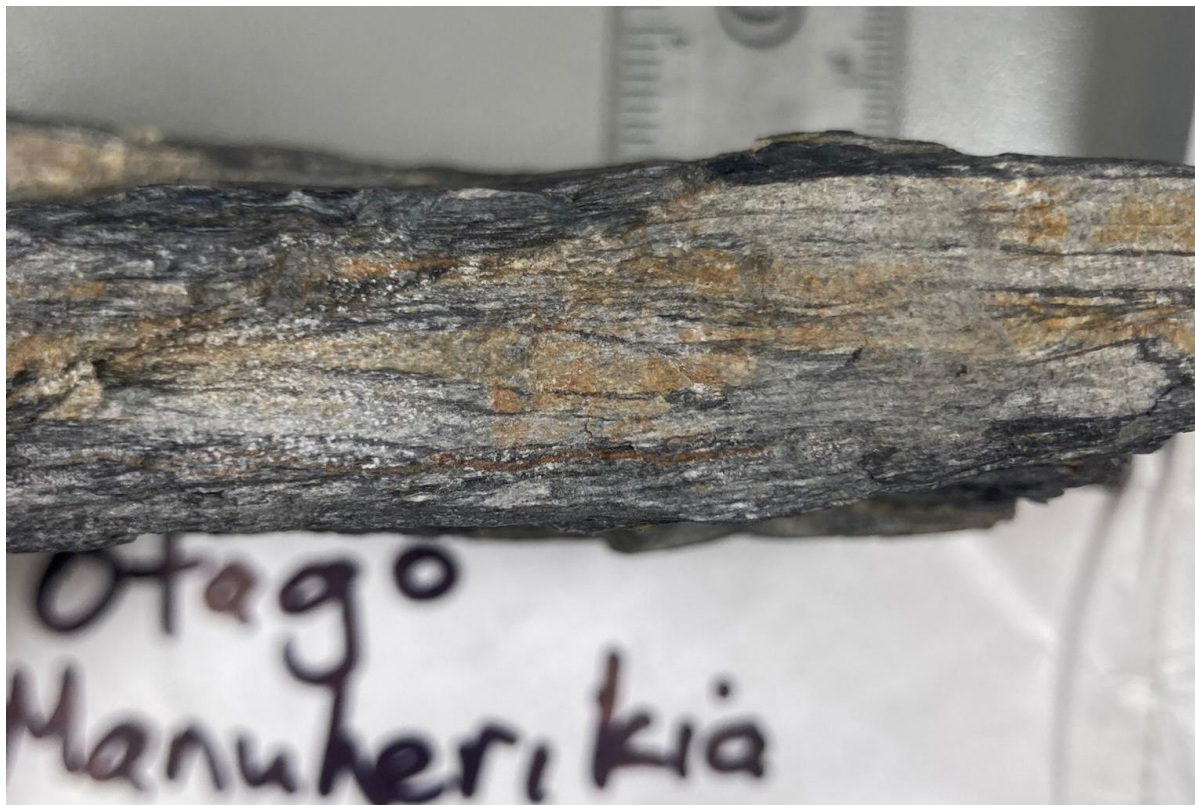
Figure 4.3: Ot.Cl.1 – Otago Chlorite Schist from the Manukerikia region. Showing lighter and darker coloured domains. Brown colour is likely derived from oxidation of Fe, which is contained in chlorite, and Fe-oxides.
