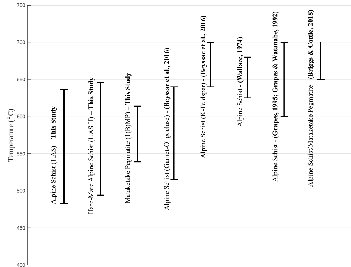
Figure 6.3 Recorded and proposed temperatures in literature for rock samples within the Mataketake Range and surrounding regions. From left to right: 1) This Study - Alpine Schist, (483-636°C), temperatures obtained from Ti-in-biotite geothermometer, 2) This Study - Alpine Schist (Hare-Mare region), (494-646°C) temperatures obtained from Ti-in-biotite geothermometer, 3) This Study - Mataketake Pegmatites, (539-614°C), temperatures obtained from Ti-in-biotite geothermometer, 4) Beyssac et al. (2016) - Garnet-Oligoclase zone Alpine Schist (515-640°C; Figure 6.4), temperatures obtained from RSCM thermometry (Section 2.2.1), 5) Beyssac et al. (2016) - Extrapolation of metamorphic temperatures starting at 640°C in the Southern region of Alpine Fault (Copland, Karangarua, Moeraki, Otoko & Haast (Locations in Figure 6.4), see Figure 10 in Beyssac et al. (2016), temperatures obtained from RSCM thermometry (Section 2.2.1), 6) Wallace (1974), (625-680°C) - Proposed metamorphic temperatures in Mataketake Range and “similar” conditions to formation of pegmatites, temperatures obtained from experimentally calibrated reactions and petrology, 7) Grapes and Watanabe (1992) & Grapes (1995), (600-700°C) - Peak metamorphic temperatures for Alpine Schist in the Franz-Josef-Fox area (20-30km northeast of Copland (see Figure 6 in Beyssac et al. (2016)), & 8) Briggs and Cottle (2018) - Alpine Schist temperatures of “at least 650°C” to facilitate partial melting, no upper bound given.
