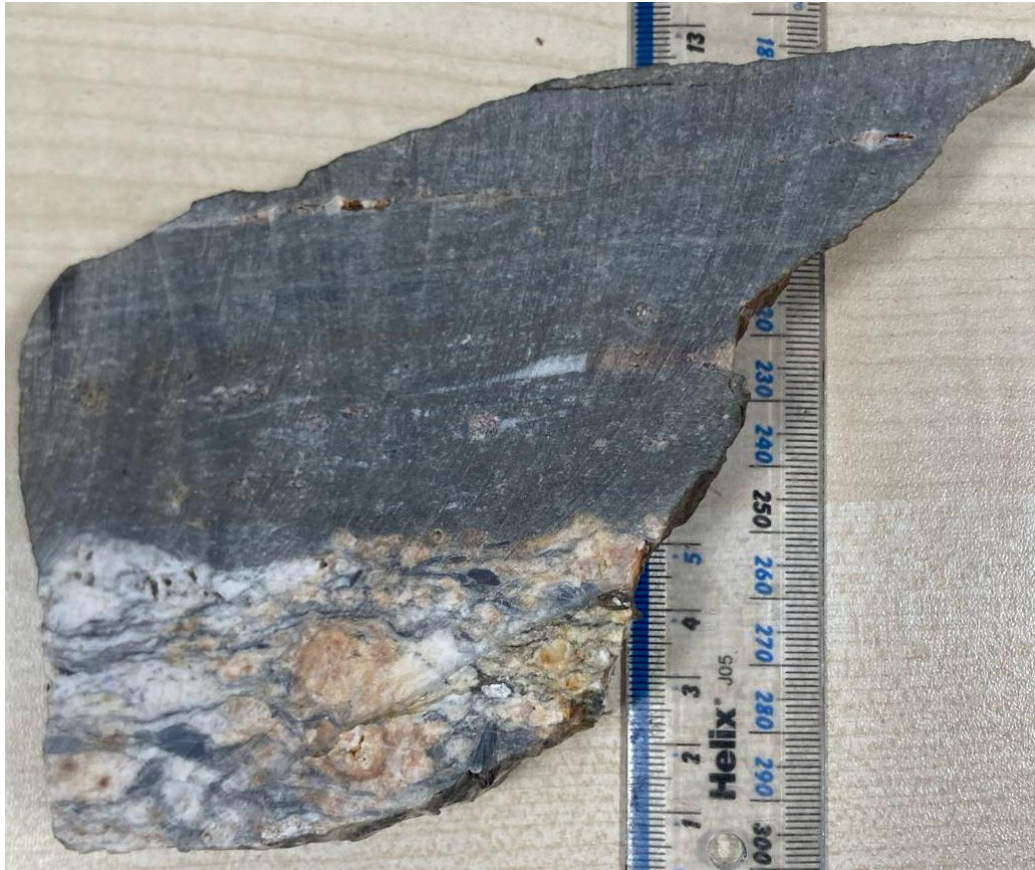
Figure 4.25: 1.AS (top) & 1(B)MP (bottom) Hand Specimen. Texturally distinct from the earlier schist/gneiss samples, with a general dark grey tone. Variation in colour reflects mineralogical changes, significantly, the relative enrichment/depletion of quartz ribbons. Garnet porphyroblasts are visible, and their pressure shadows are dominated by lighter coloured, translucent quartz. The pegmatite exists at the bottom (1(B)MP), and is described later (Section 4.3). This hand specimen was cut into three sections: 1.AS (comprising solely the Alpine Schist), 1.AS.MP.B (comprising both the schist and pegmatite), and 1(B)MP (comprising solely pegmatite).
