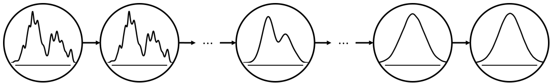
Figure 3.1: The forward process perturbs the original data distribution by gradually adding noise to training samples through a sequence of distribution transitions over multiple timesteps. Each timestep in the chain is denoted by a circle.
