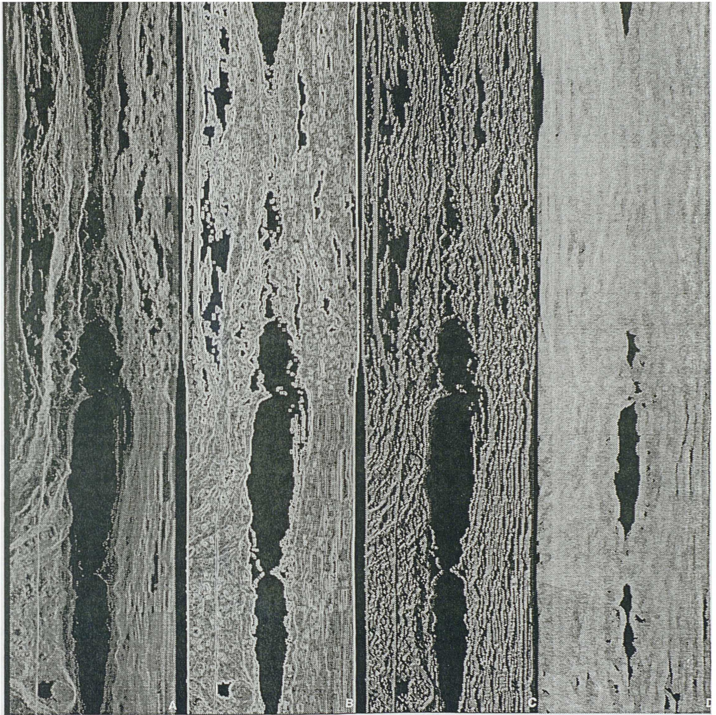
Figure 7.10 Image 4 (scale of all images is 6×24 km): (a) original grey scale image, gamma = 4.0; (b) Sobel derived edge strength image, gamma 4.0; (c) Sobel derived edge orientation image; and (d) accumulator array after first pass of transform, negatively contrasting aspect, 50° arc length, 5 radii (11-15 pixels), IT = DN 30, gamma 7.0.
