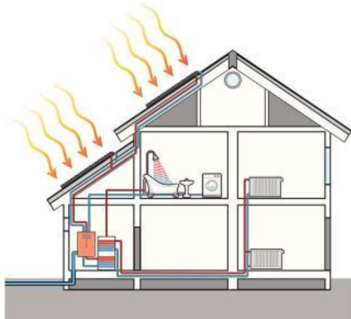
Figure C4: Diagram of house with solar panels and a solar electric boiler (Source: iStock)
