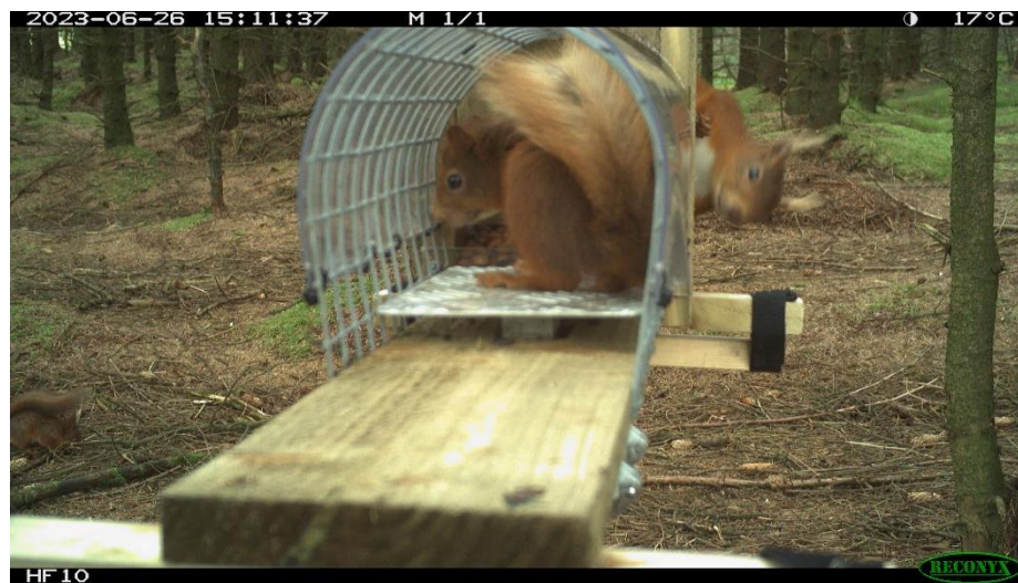
Figure 6.2. A red squirrel feeder with integrated automatic weighing scales, designed to record the body weights of red squirrels that feed from it (a). The weights, together with the date and time they were recorded, were stored on an SD card. Animals using the feeder were identified from photos and videos recorded by a Reconyx™ HS2X camera focused on the entrance of the feeder (b). Although multiple red squirrels were recorded around the feeders, the weighing platform and tunnel size meant that no more than one individual was ever recorded on the weighing platform at one time.
