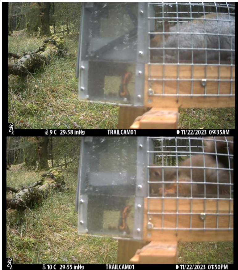
Figure 6.3. A grey squirrel selective feeder based on body weight (a). When a passive infrared sensor detected movement, the weighing platform was activated. If the weight was at least 450 g, the electronic bait door opened and stayed open for as long as the weight was maintained on the platform. The feeder entrance was monitored using a Browning™ Dark Ops Pro X 1080 camera trap, set to record one photo and one 10 second video per trigger, to identify animals using the feeder.
