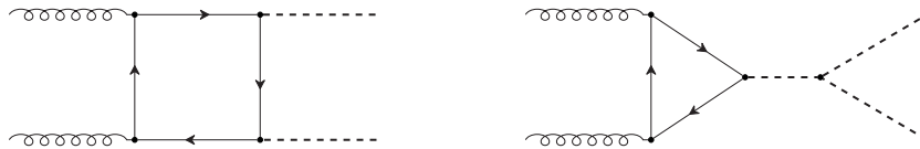
Figure 1.1: Example 1-loop (LO) box- and triangle-type diagrams contributing to HH -production in the dominant gluon fusion channel. Note the appearance at the leading order of the Higgs cubic self-coupling in the triangle-type diagrams.
