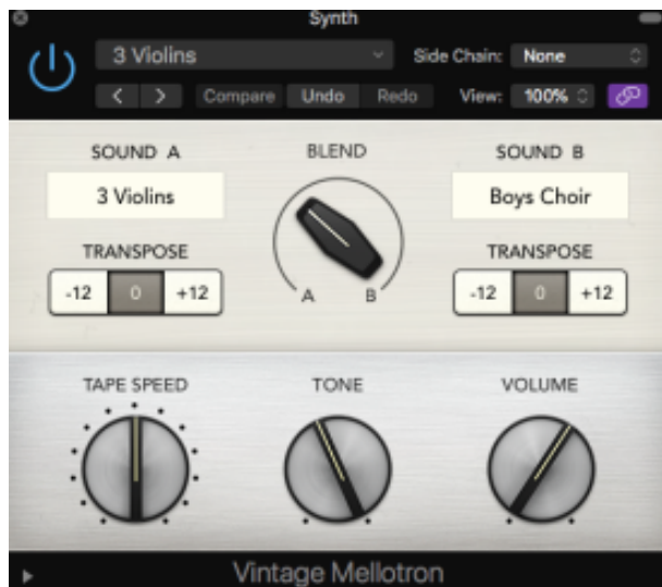
Fig.6. Settings for Logic Pro X's virtual instrument, 'Vintage Mellotron', which emulates the tape-based instrument. A string setting ('3 Violins') is selected to blend with the real string instruments in the orchestra, whilst a choral sample is also selected to add an airy timbre to the sound. The violin sample (sound A) is favoured, as indicated by the 'blend' knob, showing a c.60% bias against the choral sample (sound B). The tone knob is adjusted to control the higher frequencies, so that the instrument is not so apparent when placed in context in the texture. A tremolo effect is occasionally applied to this virtual instrument; quite different from a string instrument's tremolo, this common guitar/synthesiser effect 'ducks' the volume of the instrument at user-defined intervals. For instance, around 3'00", the effect is sped up rapidly, to mimic beating; actually, it masks beating in other instruments, adding to the confusing sonic palette.
