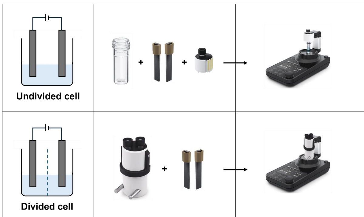
Figure 6.1: The undivided cell set up features a 10 mL glass vial with a stirrer bar, into which is placed the reaction mixture. Two electrodes are installed in the Electrasyn cap, which is then screwed onto the reaction vial. This unit is then connected to the Electrasyn and the reaction can start. The divided cell setup uses the IKA Pro-Divide, which features two PTFE chambers separated by a glass frit (pore size 10-16 \mu\text{m} ). The reaction mixture is placed inside each of the chambers (3-7 mL) and electrodes are installed. This unit can then be connected to the Electrasyn and the reaction can start.
