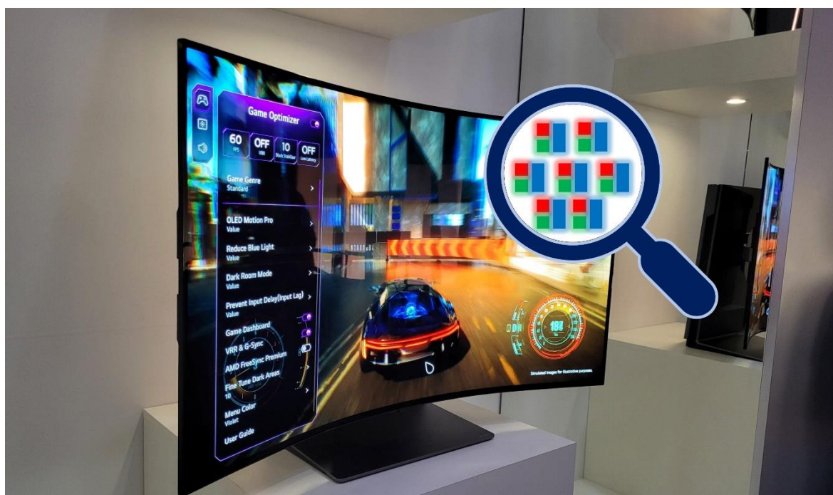
Figure 1.1. OLED v. Zoom in: the individual pixels. Typically, the blue pixel has a bigger size to reduce the blue OLED lifetime problem.
