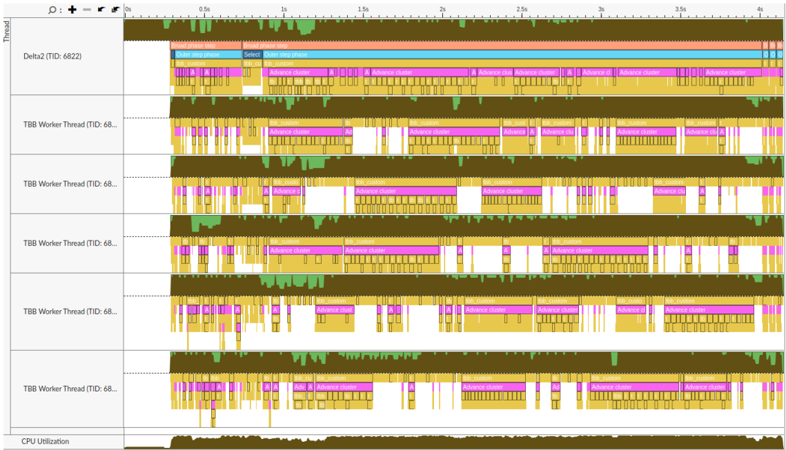
Figure 4.21: VTune analysis of the hopper’s first five compute steps using six threads. The steps are of extremely varying length. The long step has an elongated time step selection phase (dark blue), followed by the individual cluster updates.
