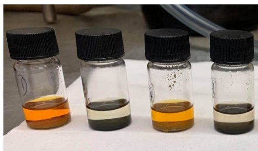
Figure 5.15: Methyl red with catalysts in toluene. From left to right: \text{Ag}/\alpha\text{-Al}_2\text{O}_3 (from Chapter 4), \text{Ag}/\gamma\text{-Al}_2\text{O}_3 (from Chapter 4), \text{Cs-Ag}/\alpha\text{-Al}_2\text{O}_3 , \text{Cs-Ag}/\gamma\text{-Al}_2\text{O}_3 .
