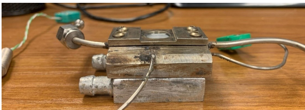
Figure 3.14: The cell is connected to the water-cooling system by epoxy.
