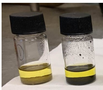
Figure 4.38: Methyl yellow with catalysts in toluene. Left is \text{Ag}/\alpha\text{-Al}_2\text{O}_3 and right is \text{Ag}/\gamma\text{-Al}_2\text{O}_3 .
