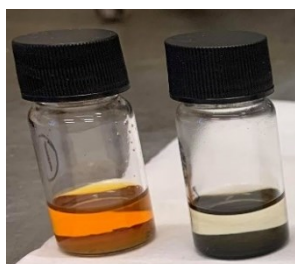
Figure 4.39: Methyl red with catalysts in toluene. Left is \text{Ag}/\alpha\text{-Al}_2\text{O}_3 and right is \text{Ag}/\gamma\text{-Al}_2\text{O}_3 .
