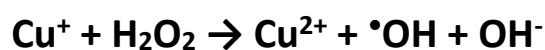
Figure 3: The Fenton reaction of Cu + with H 2 O 2 to form the hydroxide radical, • OH.
