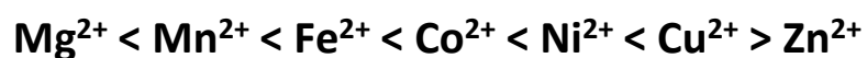
Figure 1: The Irving-Williams series of the stability of complexes formed by metal ions.
