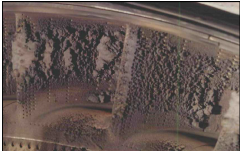
Figure 7.29: Two neighbouring NGVs taken from an engine on the 1982 British Airways Flight 9, showing the depositions of volcanic ash from Mount Galunggung. Image taken from [7].
